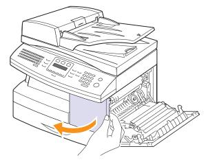
**3** Turn the cartridge locking lever upwards to release the toner cartridge.
