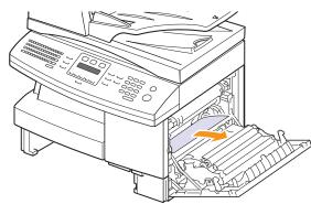
**5** Close the cover and insert the paper Tray. Lower the rear part of the Tray to align the rear edge with the corresponding slot of the machine, then insert it completely.
