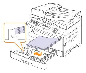
2 After loading paper, set the paper type and size for the multipurpose tray. See page 5.8 for copying and faxing or the **Software Section** for PC-printing.
