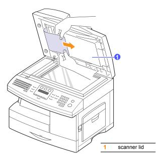
3 Close the scanner lid. Then load the removed pages back into the ADF.
