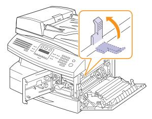
6 Turn the Jam Remove Lever back to the original position.
