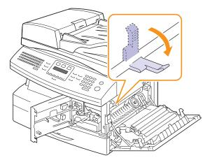
4 Turn the Jam Remove Lever in the direction of the arrow to move the paper to the exit area, then gently pull the paper out through the exit area.
