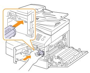
7 Reinstall the toner cartridge, and then lock the lever.
