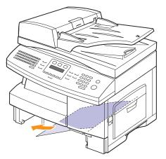
Once you remove the jammed paper here, open the side cover and then close it to clear the "Paper Jam0" message on the display.
