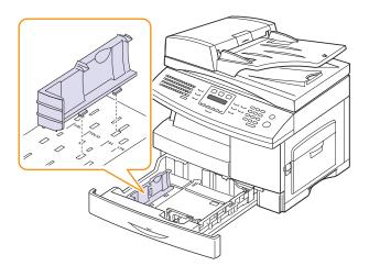
2 After inserting paper into the tray, while pinching the paper width guide as shown, move it toward the stack of paper until it lightly touches the side of the stack. Do not press the guide too tightly to the edge of the paper; the guide may bend the paper.
