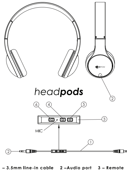
1 - 3.5mm line-in cable 2 - Audio port 3 - Remote
