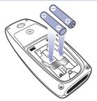
Replace the battery cover: hook the two plastic clips into place first, then lower and screw the cover into place. Finally, screw the belt clip on. You can use a coin, e.g. 10p piece if
