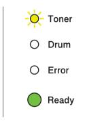
If the LEDs show this indication, the toner is low. Buy a new toner cartridge and have it ready before you get a Replace Toner indication. To replace the toner cartridge, see *Replacing the toner cartridge* on page 71.
