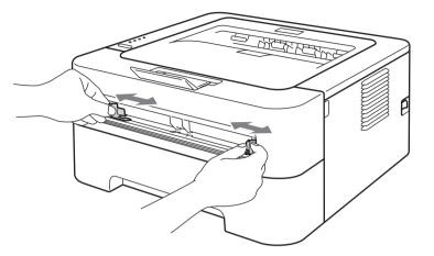
Using both hands, put one piece of paper in the manual feed slot until the front edge of the paper touches the paper feed roller. When you feel the machine pull in the paper, let go.
