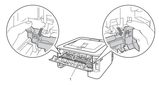
8 Using both hands, gently pull the jammed paper out of the fuser unit.
