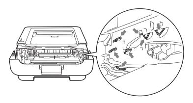
Clean the primary corona wire inside the drum unit by gently sliding the green tab from right to left and left to right several times.
