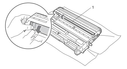
When you have found the mark on the drum that matches the print sample, wipe the surface of the OPC drum with a dry cotton swab until the dust or glue on the surface comes off.
