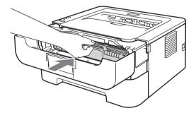
8 Press and hold down **Go** for about 4 seconds until all the LEDs light up. Once all four LEDs are lit, release **Go**.
