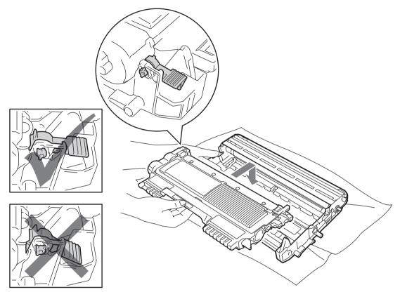
(B) Open the front cover. Put the drum unit and toner cartridge assembly back into the machine.
