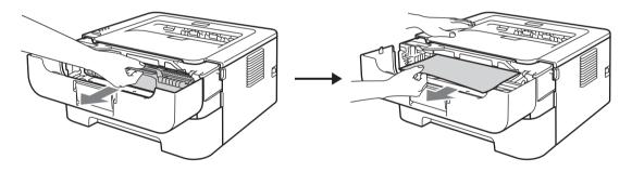
If you cannot remove the drum unit and toner cartridge assembly easily, do not use extra force. Instead, go to step ④.
