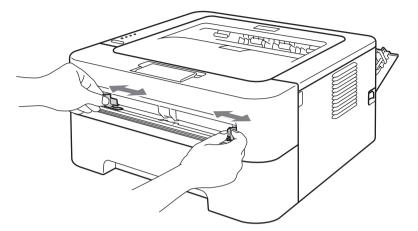
8 Using both hands, put one piece of A4 or Letter size paper in the manual feed slot until the top edge of the paper touches the paper feed roller. When you feel the machine pull in the paper, let go. The machine will start the Drum Cleaning process. The **Ready** LED flashes during the Drum Cleaning process.
