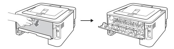
Pull down the tabs at the left and right hand sides to open the fuser cover (1).
