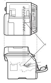
4 Put the drum unit and toner cartridge assembly back in the machine.
