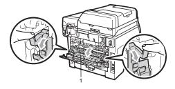
6 Pull the jammed paper out of the fuser unit.
