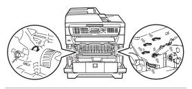
6 Put the drum unit and toner cartridge assembly back in the machine.
