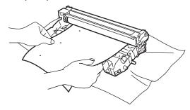
5 Turn the drum unit gear by hand while looking at the surface of the OPC drum (1).
