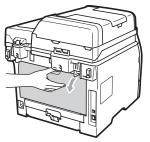
5 Pull the tabs at the left and right hand sides toward you to open the fuser cover (1).
