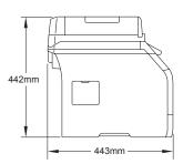
Weight With Drum/Toner Unit: 15.7 kg (MFC-8380DN)
