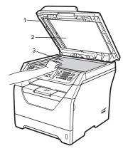
In the ADF unit, clean the white bar (1) and the scanner glass strip (2) underneath it with a soft lint-free cloth moistened with water.
