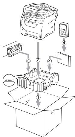
9 Take the two styrofoam pieces and match the front of the machine to the "FRONT" mark on one of the styrofoam pieces, and the back of the machine to the "REAR" mark on the other styrofoam piece (5). Coil the cables and place them and the Quick Setup Guide in the spaces provided as shown below (6).
