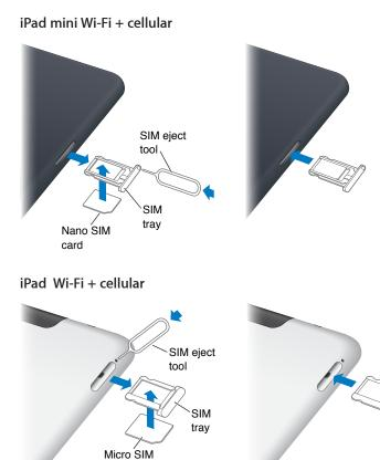
**Open the SIM tray:** Insert the tip of the SIM eject tool into the hole on the SIM tray. Press firmly and push the tool straight in until the tray pops out. Pull out the SIM tray to install or replace the SIM card. If you don't have a SIM eject tool, you may be able to use the end of a small paper clip.
