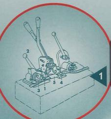
Take the leading end of the strapping, and secure it under the gripper foot (1) by bringing the handle (2) down. Pass the strapping under the cutting block (4) and round the parcel and over foot (3) and (4) then feed it into the split of the windlass (5).
