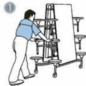
With travel lock engaged push from the seats as shown.
