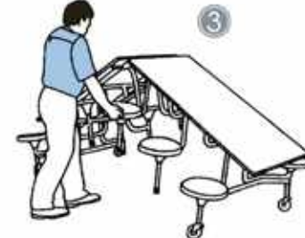
Continue opening by pressing down with both hands on the centre stools.
