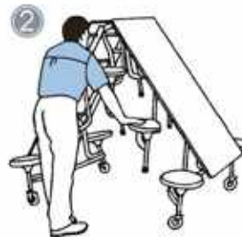
Continue opening by pressing down with both hands on the middle stools.
