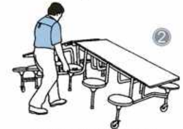
Continue to lift using centre stools.
