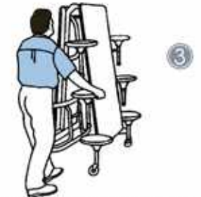
Using the middle stools push together to engage travel lock.
