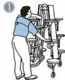
With your left hand pushing down the travel lock, push apart the stool unit with your right hand on the middle stool.
