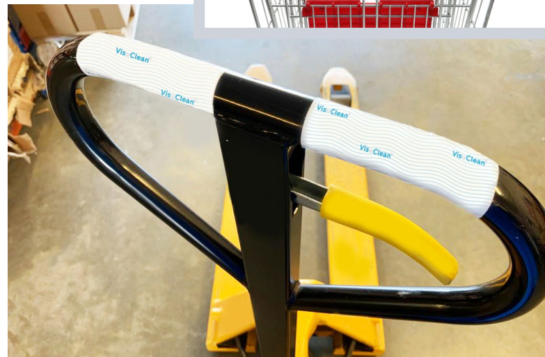
Please note: Handles on pallet trucks or trolleys must be symmetrical to prevent creasing.
