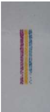
Fig. 24: Colour sample released by automatic print head cleaning
