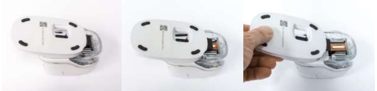
Fig. 27: Clean print head with wiper
