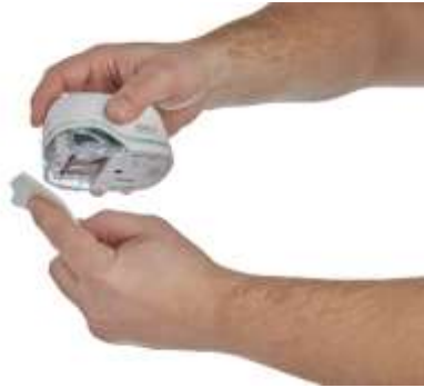
Fig. 28: Clean print head with damp cloth
