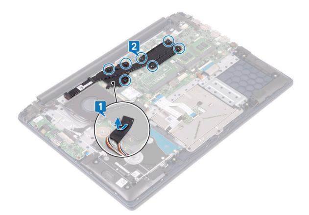
c Lift the heatsink away from the system board .
