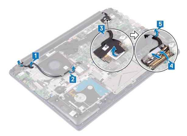
f Remove the five (M2.5x5) screws that secure the display hinges to the palmrest and keyboard assembly .
