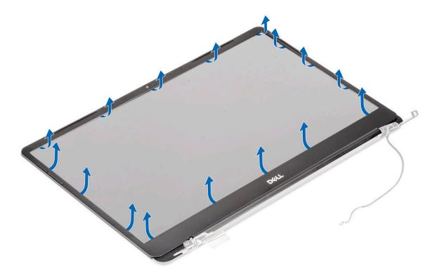
b Lift the display bezel away from the display assembly.
