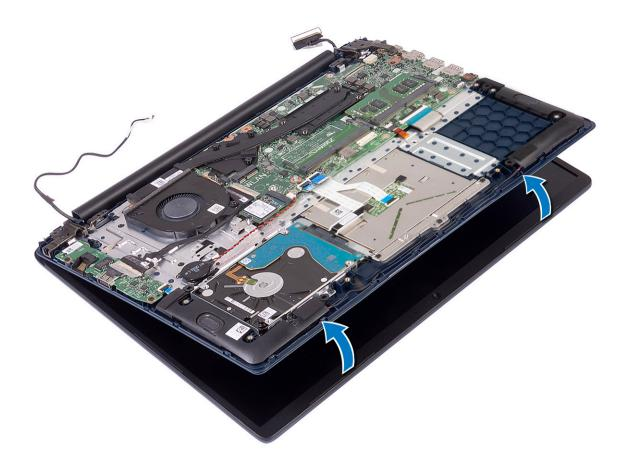
h Lift the display assembly away from the palm-rest and keyboard assembly.
