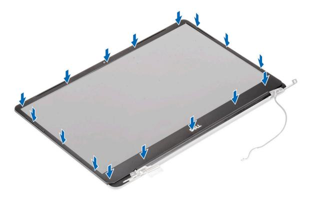
b Press the edges of the display bezel until it clicks onto the display assembly.
