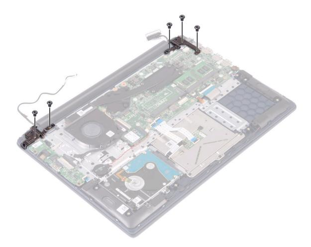
g Open the display assembly at an angle of 90 degrees.
