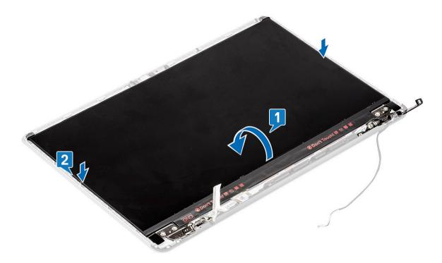
e Replace the 2 (M2x3) and 8 (M2x2.5) screws to secure the display panel to the display assembly [1, 2].
