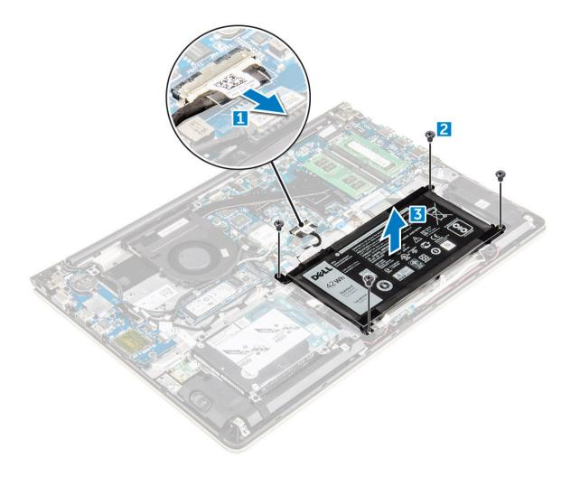
Figure 7. Removing the battery
