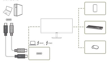
If multiple source devices are connected to the PC, the many cables around the PC may look messy. Connecting the devices directly to the product will resolve such inconvenience.
