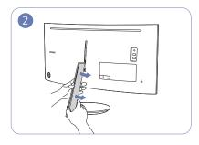
Grab the stand with one hand and use the thumb on your other hand to remove the COVER-STAND NECK LEFT in the direction of the arrow.
