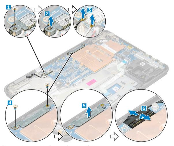
Disconnect the sensor cable, and turn over the computer [1, 2]
