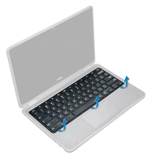
NOTE: Carefully pull the keyboard connector through the gap in the palm rest.
