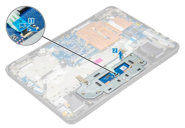
4 Remove the screws (M2.0x3.0, M.2.0x2.0) that secure the metal bracket to the touchpad on the computer.
