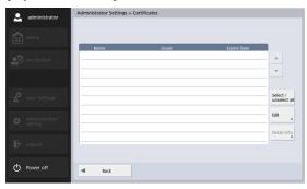
The certificates imported to the ScanFront for using the following transmission protocols is displayed. LDAP, SMTPS, STARTTLS, FTPS (Explicit mode /Implicit mode), and WebDAV over SSL
