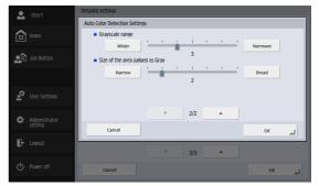
This is enabled when Auto Color Detection is selected, and allows you to configure the following detection settings for determining whether to scan a document in color or black and white.
