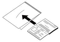
3. Load the document with the sealed end of the carrier sheet as the leading edge and the page you want to scan facing down.
