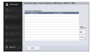
Displays the communities for which the SNMP traps are configured.
