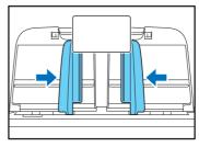
Place the card face down with the top edge at the bottom of the tray.
