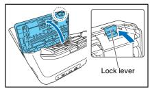
**4.** Pull out the jammed document in the direction that seems the easiest to remove it.
