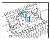
3. Pull the left lever that secures the retard roller to the scanner, and remove the roller.
