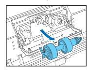
**4.** Remove any dirt from the roller using a cloth that has been soaked in water and thoroughly wrung out.
