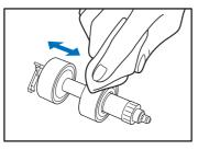
Install the cleaned retard roller by inserting the right side first.
