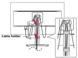
Rotate Set(Pivot) and put connectors. It is easy to put connectors and manage cables using cable holder.
