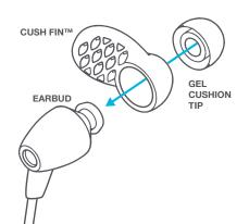
Rotate Cush Fins to desired position.
