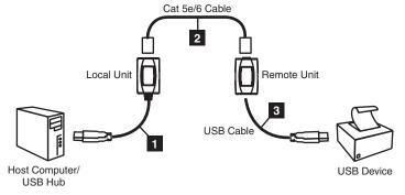
Note: Diagram shows the B202-150. Connections will be the same for the B202-150-WP, except separate USB A/B device cables will be needed.
