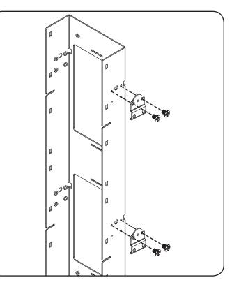
**Step 2** Using (2) M4 x 12 mm pan head screws, attach (2) mounting buttons to the mounting brackets.
