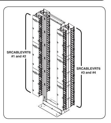
Note: SRCABLEVRT6 is shown. The cable tray frames and doors of the SRCABLEVRT12 are wider, but installation is identical.
