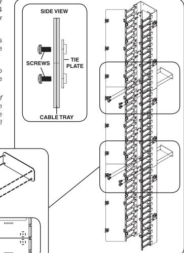
**Step 7** (Optional) Repeat Steps 1-6 to install another set of cable trays on the other side of the rack. (A single-depth installation on both sides of the rack requires 2 x SRCABLEVRT6 or SRCABLEVRT12.)
