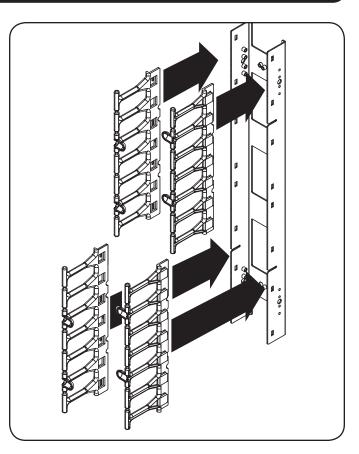
**Step 4** Slide (6) door hinges over the edges of (3) cable tray door straps, then fasten the door straps to the cable guides via the door hinges' C clasps. After installation, you can release the C clasps on one side of the cable tray door straps to open them from either side.
