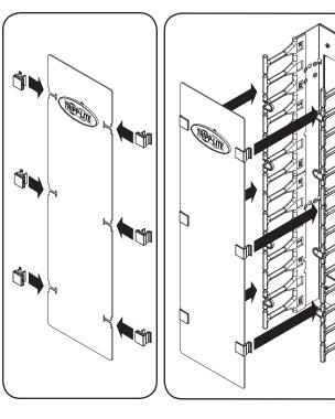
Step 5 Align the mounting buttons with the toolless mounting slots on the side of the rack. Insert the mounting buttons through the slots and slide the cable tray downward until secure. Use (4) M4 x 12 mm pan head screws inside of the rack rail to fasten the cable tray in place.
