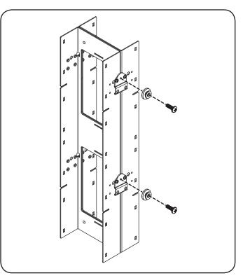
**Step 3** Attach (8) cable guides to the cable tray frames. The cable guides slide over the edges of the cable tray frames to form a tight attachment.
