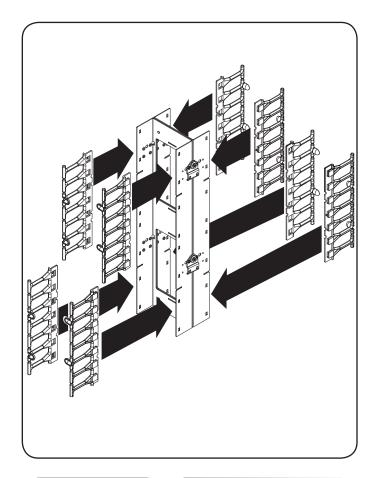
**Step 4** Slide (6) door hinges over the edge of (1) cable tray door, then fasten the door to the cable guides via the door hinges' C clasps. Repeat for the other cable tray. After installation, you can release the C clasps on one side of the cable tray door to open it from either side.
