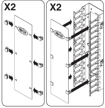
Step 5 Align the mounting buttons with the toolless mounting slots on the side of the rack. Insert the mounting buttons through the slots and slide the cable trays downward until secure. Use (4) M4 x 12 mm pan head screws inside of the rack rail to fasten the cable trays in place.
