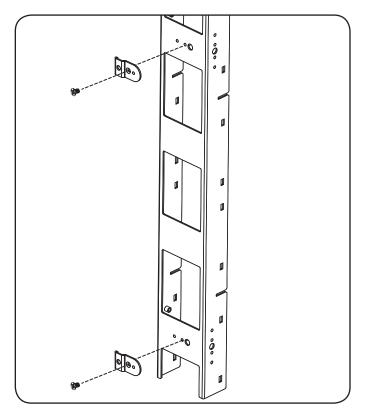
**Step 2** Using (2) M4 x 12 mm pan head screws, attach (2) mounting buttons to the mounting brackets.
