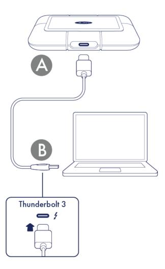
Alternatively, you can connect Rugged SSD Pro to a USB-3.1 Gen 1/Gen 2 (USB-C) port. Transfer speeds vary (see Cables and Connectors).
