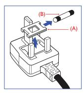
This apparatus is supplied with an approved moulded 13A plug. To change a fuse in this type of plug proceed as follows:
