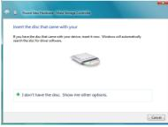
**NOTE:** If automatic installation fails, you may need to point the driver installation wizard to the driver location on the CD, manually: "IO \ MOSCHIP \ MCS99xx"
