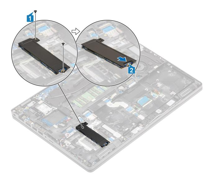
2. Turn the metal bracket over and detach the ssd module from the thermal pad on the metal bracket.
