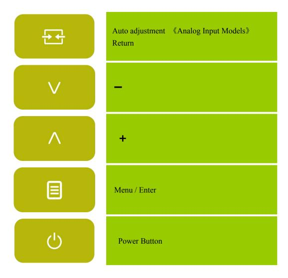
Figure.4. Control Panel Buttons
