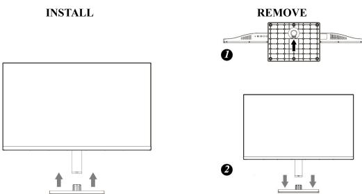
Figure.1. Installing and Removing the Base
