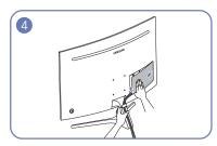
Grab the stand with one hand and use the thumb on your other hand to remove the COVER-CLEAN BACK TERMINAL in the direction of the arrow.
