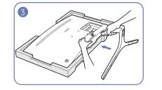
Place the protective Styrofoam (cushion) included in the package on the floor and place the product facing down on the Styrofoam, as shown in the image. If Styrofoam is unavailable, use a thick sitting mat. Hold the back of the monitor as shown in the figure. Push the assembled stand into the main body in the direction of the arrow as shown in the figure.
