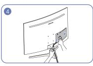
Grab the stand with one hand and use the thumb on your other hand to remove the COVER-CLEAN BACK TERMINAL in the direction of the arrow.
