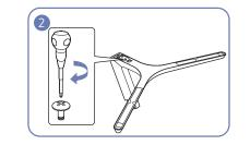
Insert the stand neck into the stand base in the direction shown in the figure.
