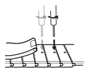
2. Remove a link from both sides of the clasp to make sure the watch face is still centred.
