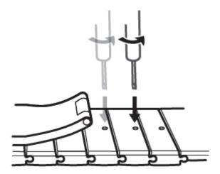
2. Remove a link from both sides of the clasp to make sure the watch face is still centered.
