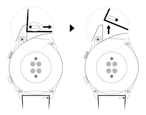
To remove a metal strap, perform the steps shown in the following figure. Follow the steps in the reverse order to install a new strap.
