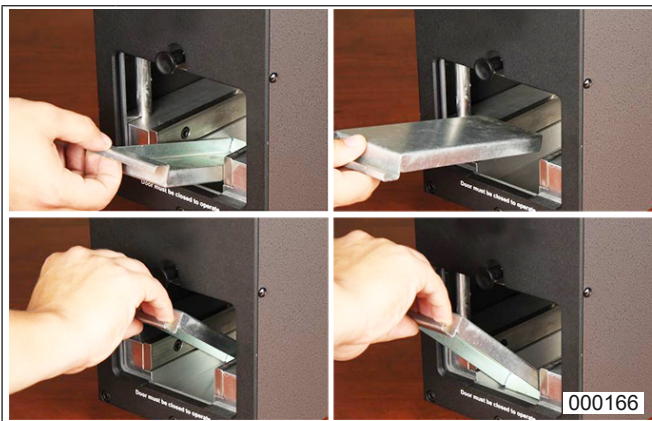
Fig. 13 Tip: Use debris tray for cleaning
