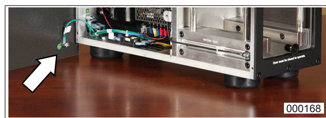
Fig.2 Open side panel with ground cable
