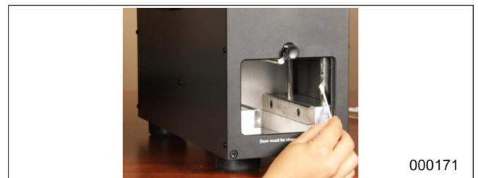
Fig. 15 Greasing the Vertical Crusher Slide Rails
