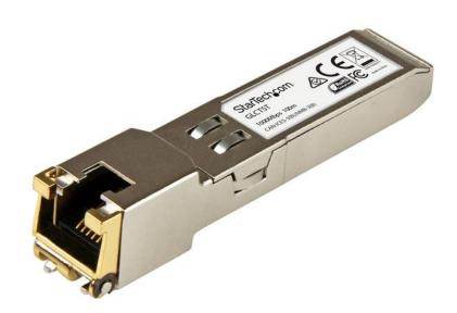
The 10050-ST is an Extreme Networks 10050 compatible copper transceiver module that has been designed, programmed and tested to work with Extreme Networks brand switches and routers. It delivers dependable 1 GbE connectivity over copper cable, for 1000Base-T compliant networks, with a maximum distance of up to 100 m (328 ft).
