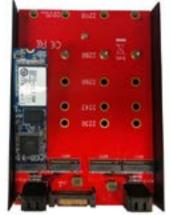
Note: The connector on your M.2 SSD is keyed so the drive will only fit one way.
