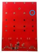
4. (Only required if the drive installation screw and standoff requires relocating) Remove the SSD installation standoff, and reseat it into the drive installation hole that matches your SSD. Replace the nut on the reverse side and secure it into place using a small phillip's head screw driver.
