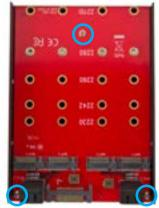
Slide the M.2 connector on the SSD into the M.2 receprical connector on the 35S24M2NGFF.
