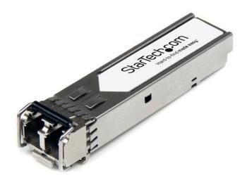
The AR-SFP-10G-LR-ST is an Arista Networks SFP-10G-LR compatible fiber transceiver module that has been designed, programmed and tested to work with Arista Networks brand switches and routers. It delivers dependable 10 GbE connectivity over fiber cable, for 10GBase-LR compliant networks, with a maximum distance of up to 10 km (6.2 mi).
