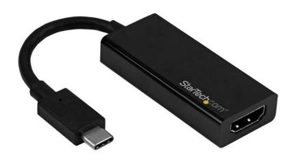
This USB-C<sup>TM</sup> to HDMI® adapter lets you output HDMI video and audio from a USB Type-C<sup>TM</sup> device, such as a USB-C equipped MacBook, with support for Ultra HD 4K at 60 Hz. This adapter works with USB-C devices that pass a DisplayPort video signal, and it's also compatible with Thunderbolt<sup>TM</sup> 3 ports.
