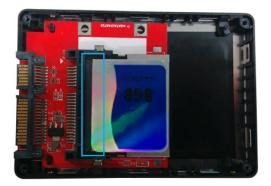
**Note:** The connector on your CFast card is keyed so the card will only fit one way.
