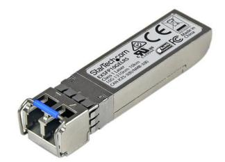
The EXSFP10GELRS is a Juniper EX-SFP-10GE-LR compatible fiber transceiver module that has been designed, programmed and tested to work with Juniper® brand switches and routers. It delivers dependable 10GbE connectivity over fiber cable, for 10GBASE-LR compliant networks, with a maximum distance of up to 10 km (6.2 mi).
