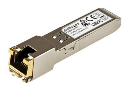
The EXSFP1GETST is a Juniper EX-SFP-1GE-T compatible copper transceiver module that has been designed, programmed and tested to work with Juniper® brand switches and routers. It delivers dependable 1 GbE connectivity over copper cable, for 10BASEBASE-T, 100BASE-TX and 1000BASE-T compliant networks, with a maximum distance of up to 100 m (328 ft.).
