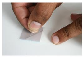
1. Remove the clear plastic backing from the compound to expose the adhesive. Removing the plastic in one quick, smooth motion will ensure that no plastic remains on the adhesive.
