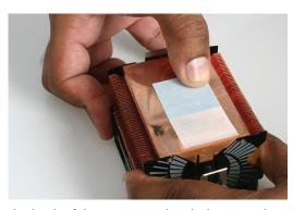
3. Smooth the back of the compound with downward pressure to ensure a consistent application.
