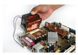
5. Install the heatsink and fan according to the instructions from the manufacturer.
