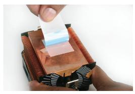
4. Using a single quick smooth motion, remove the wax paper from the compound. Ensure to remnants of wax paper remain.
