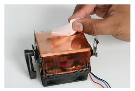
2. Place the compound (adhesive side down) to the bottom of the heatsink. Generally, affixing the pad to the center of the heatsink offers the best performance.
