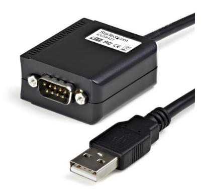
The ICUSB422 6ft Professional RS422/485 USB Serial Cable Adapter with COM Port Retention lets you connect RS422 or RS485 serial devices to your USB-enabled computer. The adapter features a 9-pin (DB9) male serial connector as well as dipswitch controls for easy port configuration, and requires minimal software.
