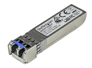
The MASFP10GBLR is a Cisco Meraki MA-SFP-10GB-LR compatible fiber transceiver module that has been designed, programmed and tested to work with Cisco Meraki<sup>™</sup> brand switches and routers. It delivers dependable 10GbE connectivity over fiber cable, for 10GBASE-LR compliant networks, with a maximum distance of up to 10 km (6.2 mi).
