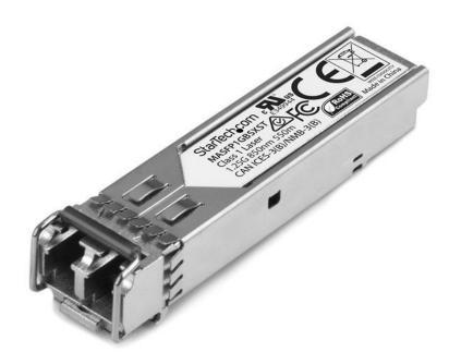
The MASFP1GBSXST is a Cisco Meraki MA-SFP-1GB-SX compatible fiber transceiver module that has been designed, programmed and tested to work with Cisco Meraki™ brand switches and routers. It delivers dependable 1GbE (1000 Mbps) connectivity over fiber cable, for 1000BASE-SX compliant networks, with a maximum distance of up to 550m (1804 ft).
