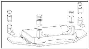
Inserting the Rubber Feet into the Legs
