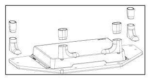
Inserting the Extenders into the Legs
