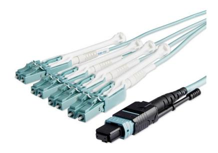
This MPO/MTP to 8x LC breakout cable lets you fan out a single 40Gbps connection from a 40GBase-SR4 QSFP+ transceiver to four 10Gbps LC SFP+ transceivers.
