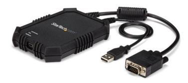
This rugged and portable USB crash cart adapter lets you turn your laptop into a portable console for accessing servers, desktops and laptops, as well as ATMs, kiosks or any computing device that features both VGA and USB ports.
