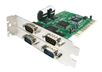
The PCI4S550N 4-port PCI Serial card turns an available PCI slot into four RS232 serial ports - a cost-effective solution for connecting any new or old serial peripheral, with support for data transfer rates of up to 115Kbps.
