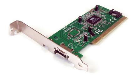
This PCI based SATA Controller Card allows you to turn a PCI slot into one internal SATA and one external SATA (eSATA) connection. Supporting SATA 150 hard drives, and data transfer rates of up to 1.5Gbps, this controller card is the perfect solution if you need an extra SATA port or want to externalize your storage.
