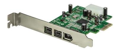
This 3 Port PCI Express FireWire adapter card can be installed in a PCI Express slot to add two IEEE1394b (FireWire 800 - 9 pin) ports and one IEEE1394a (FireWire 400 - 6 pin) port, providing broad compatibility with a wide range of FireWire devices (e.g. DV camcorders, external hard drives, digital cameras, etc.).
