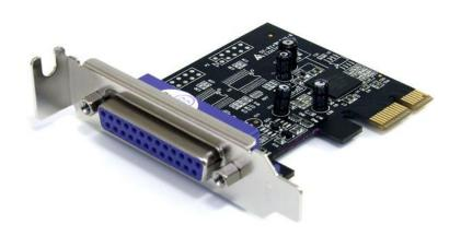
The PEX1PLP PCIe Parallel Adapter card can be installed in a PCI Express (PCIe) x1 slot, allowing you to connect EPP/ECP parallel peripherals to any computer, while relying on a native, single-chip design (Oxford OXPCIe952) that harnesses the capability of true PCI Express - ensuring maximum performance and reliability.
