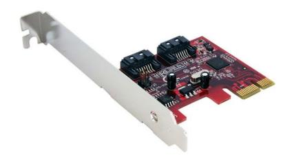
The PEXSAT32 2-Port PCI Express SATA 6 Gbps (SATA 3.0) Controller Card offers simple connectivity between a host computer and SATA 3.0 devices - a cost-effective solution for connecting high-speed storage, such as High RPM Hard Drives and Solid State Drives (SSD), which in turn allows for easier data backups and archiving.
