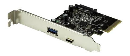
This USB 3.1 card lets you add one USB-C<sup>™</sup> port and one USB-A port to your computer, through a PCI Express slot. It enables you to upgrade your current system by adding two USB 3.1 Gen 2 ports to your computer and giving you access to data transfer speeds up to 10Gbps per port.
