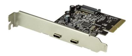
This USB 3.1 card lets you add two USB- $C^{\text{TM}}$  ports to your computer, through a PCI Express slot. It enables you to upgrade your current system by adding two USB 3.1 Gen 2 ports to your computer and giving you access to data transfer speeds up to 10Gbps.
