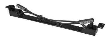
This 1U rack-mount light panel installs into any EIA-310 compliant cabinet and enables you to complete tasks inside your server rack that require lighting. The panel mounts into 1U of rack space in any standard 19 in. rack and features two adjustable gooseneck lights, each 17 in. (432 mm) in length. For easy installation, the light panel also includes a 5 ft. (1.5 m) power cord that can easily reach a PDU that's mounted inside of your rack.
